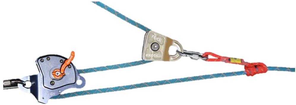
Figure 94- MPD employed in 3:1 simple pulley system.
