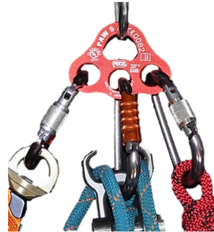
Figure 53- Rigging Plate. Keeps multiple connections organized.
