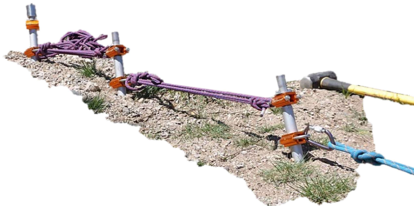
Figure 136- Picket anchor system (1-1-1 combination) constructed with a set of SMC Rescue StayK weighing 13 kg (28 lbs).
