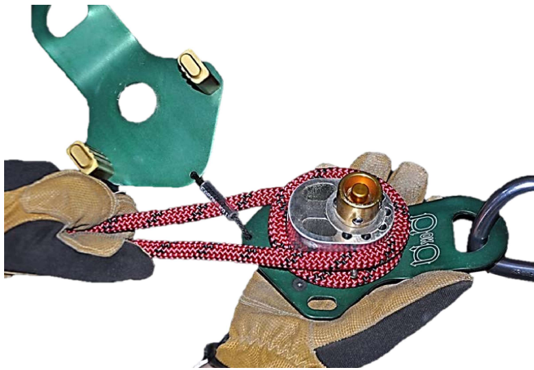
Figure 96- Loading the 540°™ Rescue Belay device with 1 1/2 complete wraps of the rope. The tether cord for the two side plates has been properly positioned between the strands.
