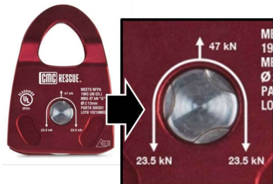
Figure 174- Pulley strength. This CMC Rescue Pulley (model 300301) has a rated breaking strength of 47 kN, which means a limit of 23.5 kN load to one strand of rope entering the pulley. Image © CMC Rescue.
