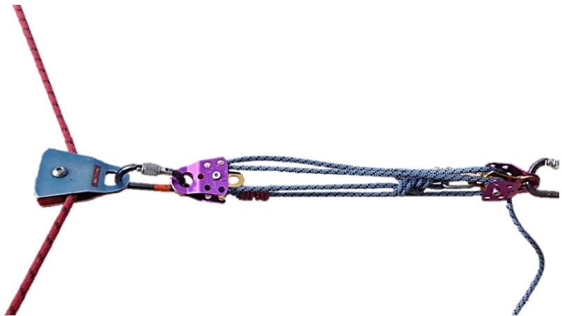
Figure 142- Directional pulley with jigger as adjustable tether.
