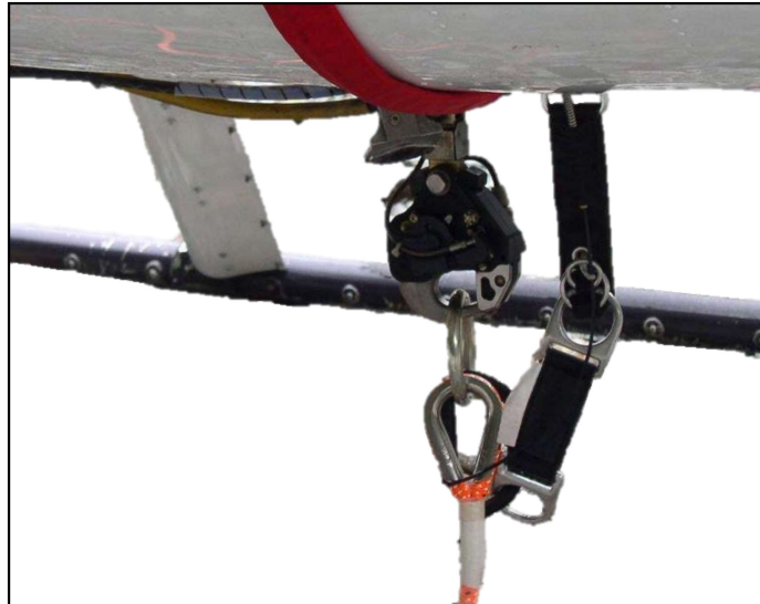
Figure 38- Anchor system. Short-haul anchor system, with releasable cargo hook serving as primary anchor point and yoke band (red) with three-ring release providing secondary anchor point. NPS photo.
