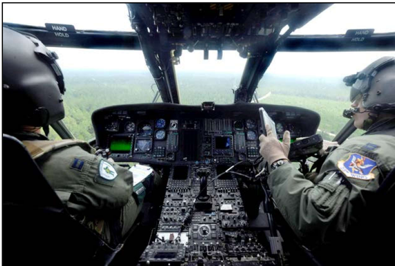
Figure 12- Two pilot configuration. Two USAF 41st Rescue Squadron pilots fly an HH-60G Pave Hawk during training at Moody Air Force Base, GA. U.S. Air Force photo, Airman 1st Class Benjamin Wiseman.
