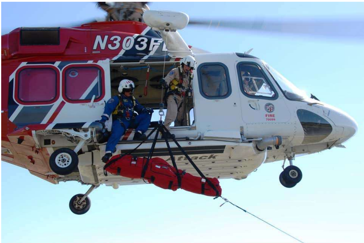
Figure 29- Hoisting with tag line. Los Angeles City Fire Department personnel aboard a twin engine AugustaWestland AW139 prepare to receive a Bauman Bag equipped with a tagline, which is controlled from the ground. Image courtesy of Los Angeles City Fire Department.
