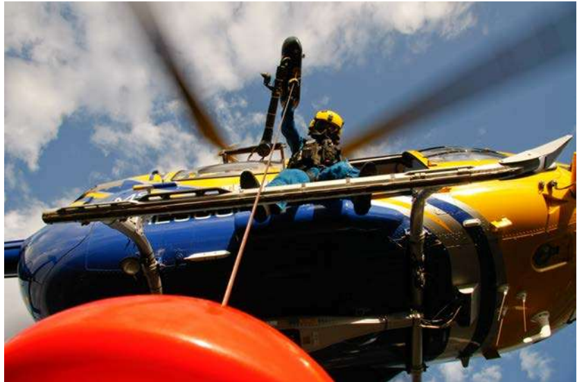
Figure 21- Hoist operator with boomed hoist. Positioned on the helicopter skid, with a secure tether to the aircraft, the hoist operator has an unobstructed view of the load. Image courtesy Travis County STAR Flight, Texas.
