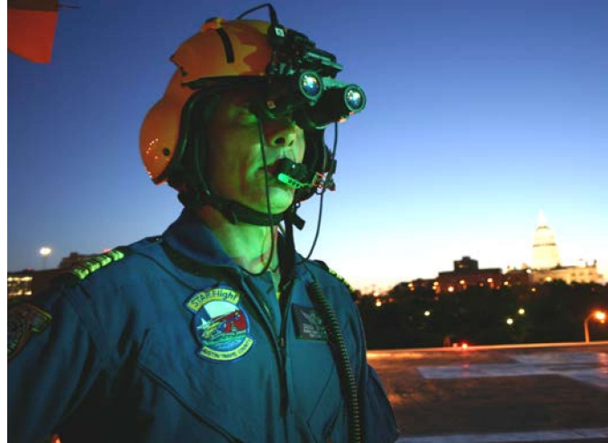
Figure 3- Night Vision Goggles. Suspended from the front of a flight crewmember’s helmet. Image courtesy Travis County STAR Flight, Texas.
