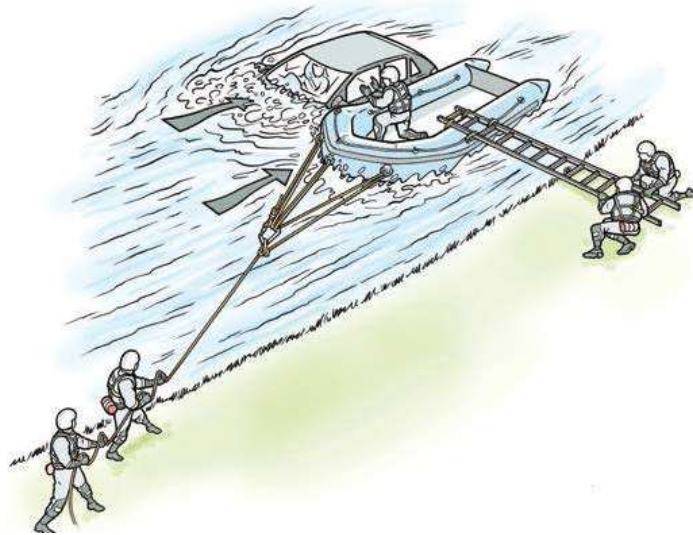
Single-point boat tether with ladder extension
